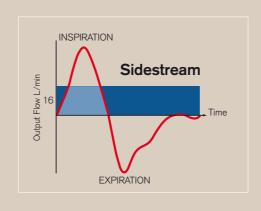
In the graphs above, the Sidestream and traditional nebulizers are compared. Both nebulizers run from the Porta-neb (6 L/min). The increased output flow from the Sidestream (16 L/min) is due to an innovative Venturi mechanism in the top of the Sidestream.
